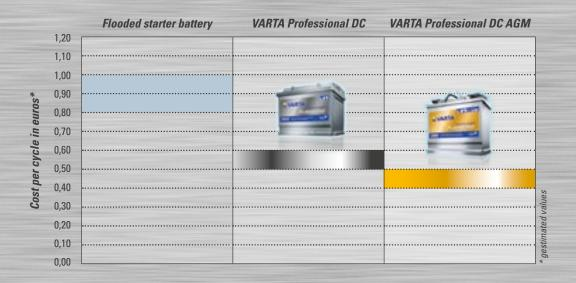
It pays to choose a battery with higher cyclic durability, a key factor in determining the battery's service life.
